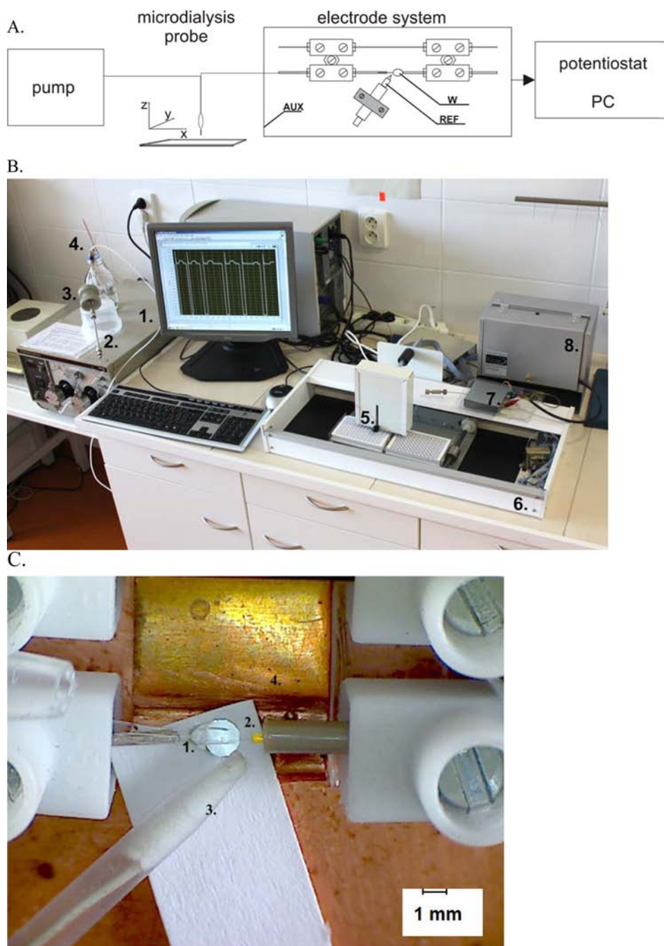
Figure 1. (A) Scheme of the arrangement used for electrochemical assay of antioxidant capacity of wine (AUX, auxiliary electrode; REF, reference electrode; W, working (carbon fiber) electrode). (B) Photograph of the apparatus (1, HPLC pump; 2, pulse damper; 3, guard column; 4, flow splitter; 5, microdialysis probe; 6, microplate positioner; 7, electrode system; 8, potentiostat). (C) Photograph of the electrode system layout (a piece of white paper was inserted below the carbon fiber electrode to make the fiber–capillary connection visible; 1, CFE; 2, carbon fiber inserted into fused silica capillary; 3, reference electrode; 4, copper foil auxiliary electrode).
